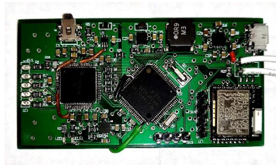
Figure 2.14: Digital photograph of miniaturized wearable design printed circuit board. Third iteration. The board was fabricated by PCBway and populated in-house. Board dimension 7.2 by 3.6 cm.
